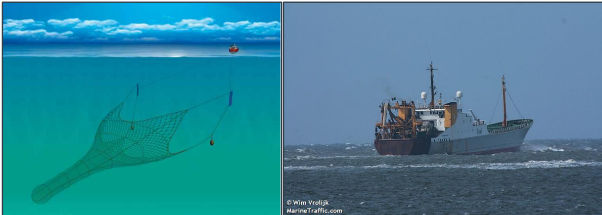
Graphic 3-24 Typical pelagic trawl vessel (Source: Seafish, 2015 and MarineTraffic.com, 2020)
